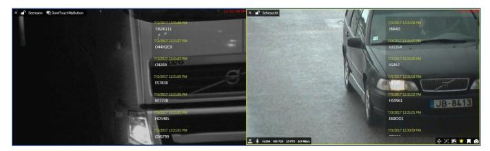
The list of the live results is cleared when you close the GANZ CORTROL Client application meaning that each time GANZ CORTROL Client starts with an empty notification pane and it gets filled as the recognition results arrive.
